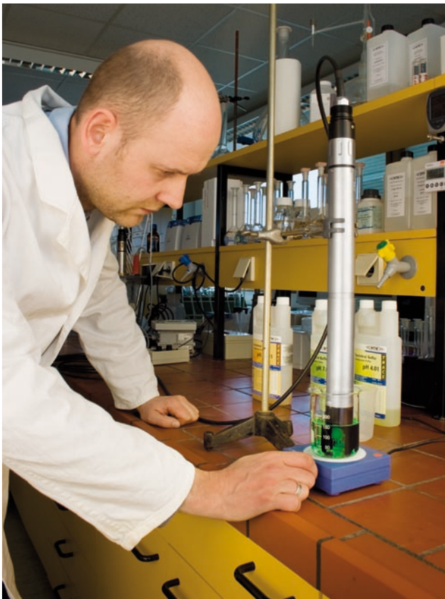
Laboratory pre-calibration of a digital sensor
